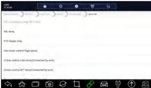
Figure 5-28 Sample Active Test Screen
